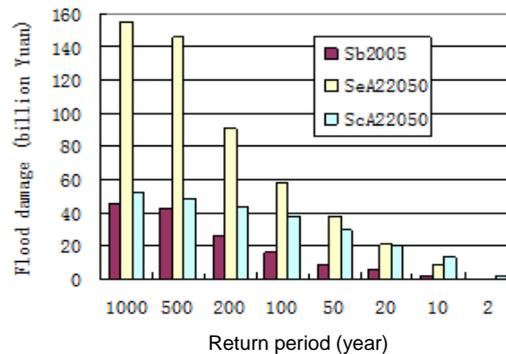
Figure 2 : Comparison of damages for the events of eight return periods in the scenario analysis
